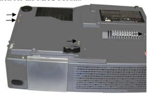
Locate the mounting points on the bottom of the projector (see arrows above for mounting point recognition).
